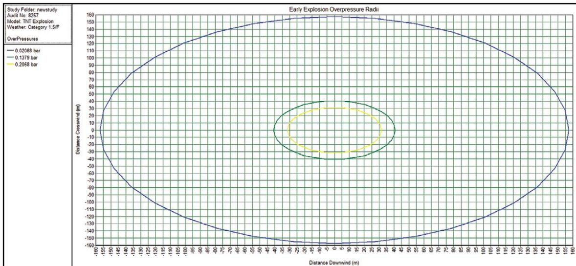
Figure 7: Overpressure plot from DNV Phast.
