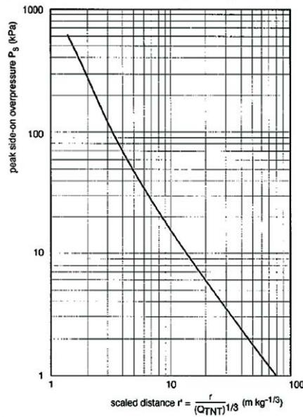
Figure 6: TNT Method – Peak Overpressure Curve.
