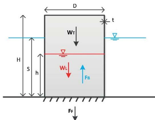
Figure 4: Schematic of the load-resistance forces considered for tank floatation.
